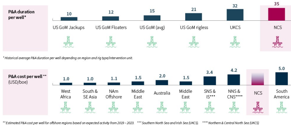
Figure 38 P&A durations and costs on the NCS compared with other basins (Rystad Energy, 2021)
