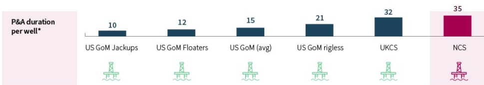
Figure 38 P&A durations and costs on the NCS compared with other basins (Rystad Energy, 2021)
