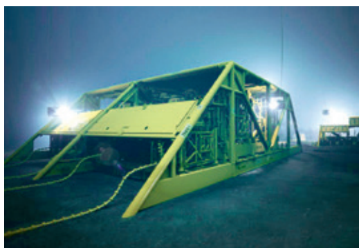
Åsgård subsea compression system. Illustration: Aker Solutions
